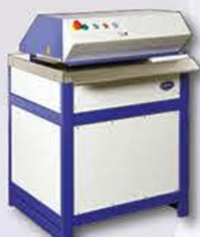
CP430S2-3PH Optimax Three Phase Cardboard Shredder Produces void fill or protective matting material
